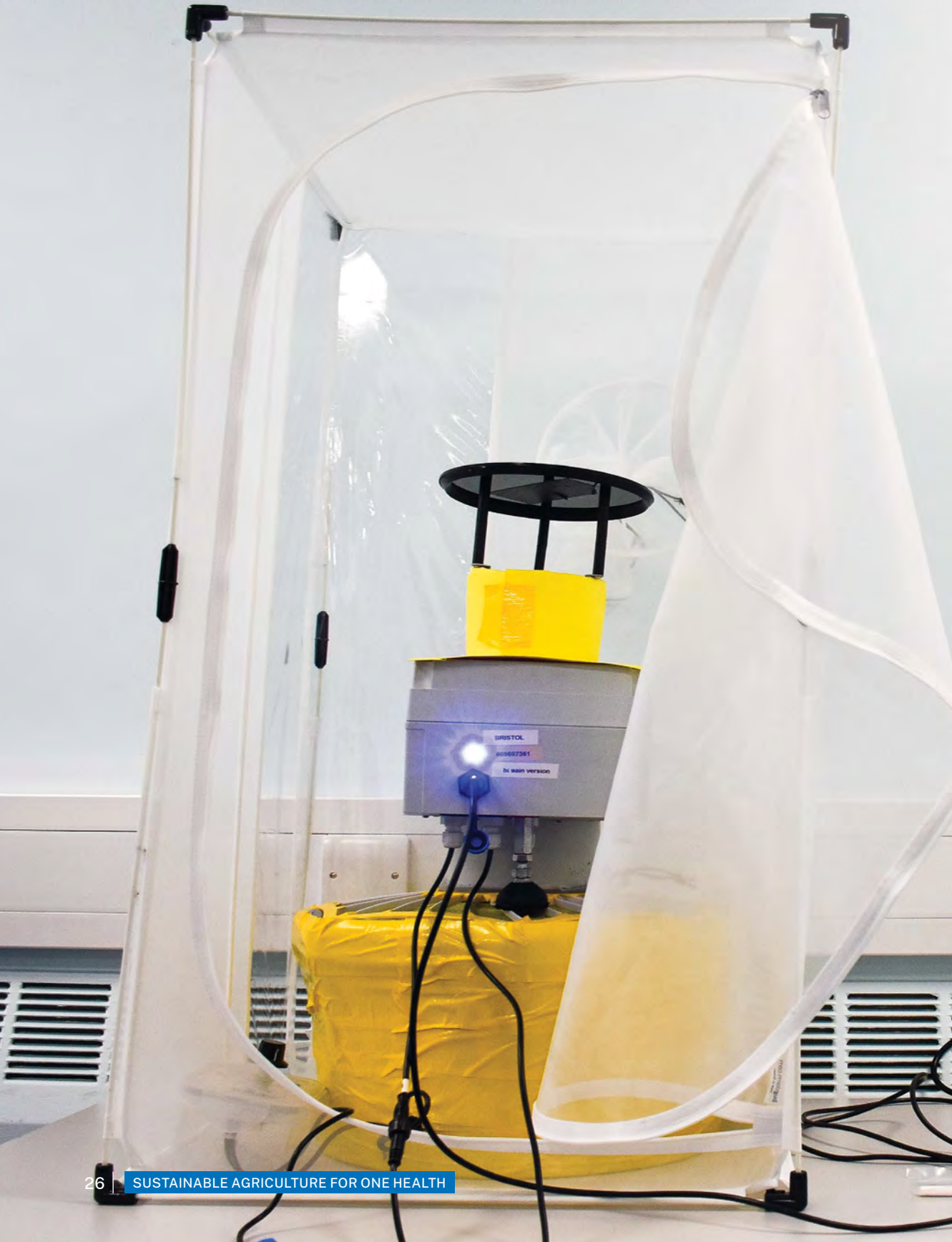
Image: The smart trap enables passive, automated and real-time detection and identification of B. tabaci
